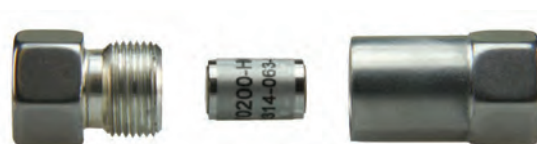
Figure 35. The 1.0mm i.d. and 2.0mm i.d. guard cartridges are for use with 1.0mm and 2.1mm i.d. analytical columns respectively, whereas the 4.0mm i.d. guard cartridges are for protection of 3.0mm and 4.6mm i.d. analytical columns. The hand-tightened holder allows for easy installation.
